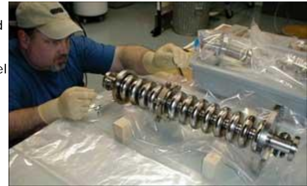
A Fermilab technician works on an array of superconducting niobium cavities at Fermilab. (Photo courtesy of Fermilab)
