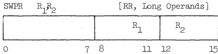
The first operand is a double word contained in an adjacent pair of general registers.  $R_1$  designates the leftmost register of the pair.  $R_1$  must be even, otherwise a specification exception is recognized. The second operand is a double word contained in a floating point register.  $R_2$  must be 0, 2, 4 or 6, otherwise a specification exception is recognized.
