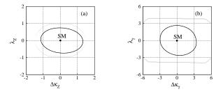
Figure 16: Contour limits on anomalous coupling parameters at the 95% CL (inner curves) and unitarity contours (outer curves) for DØ assuming  $\Lambda = 1.5$  TeV for the process  $WW/WZ \rightarrow e\nu jj$ . SM couplings have been assumed for (a)  $WW\gamma$  and (b) WWZ vertex.
