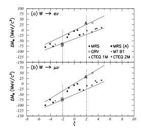
Figure 12: Correlation between  $\Delta M_W$  and  $\zeta$ , the significance of the difference between data and theory for the *W*-charge asymmetry, for various parton distribution functions for the (a)  $W \rightarrow e\nu$ - and (b)  $W \rightarrow \mu\nu$ -sample. The nominal mass measurement uses the MRSD' – parton distribution function.
