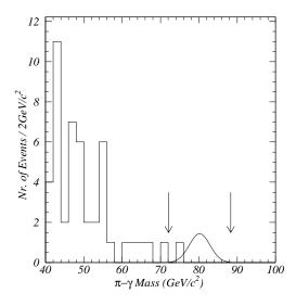
Figure 14: The CDF distribution in  $M(\pi\gamma)$  for the search for the rare decay  $W \rightarrow \pi\gamma$ . The arrows indicate the search window. The Gaussian, centered at  $M_W$ , corresponds to the 95% CL limit of 4.9 events.
