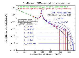
Figure 3: Double differential cross section  $d^2\sigma/dM dy$  for CDF electron and muon data combined. The open symbols are from the 88/89 data. The solid symbols correspond to the full Run I data. The curves are the theoretical predictions for different  $\Lambda_{-}$  values.
