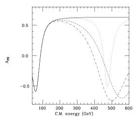
Figure 5: Parton level forward-backward asymmetry as function of center of mass energy for  $d\overline{d} \rightarrow e^+e^-$  for the SM (solid line), and for models with an additional  $Z_I$  (dashed-dotted line),  $Z_{\chi}$  (dashed line) or  $Z_{\psi}$  (dotted line) boson of 500 GeV/c<sup>2</sup> [19].
