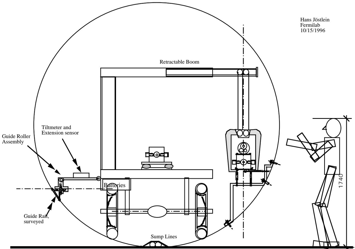
Really Large Hadron Collider, Low Field: Tunnel with Magnet Vehicle
