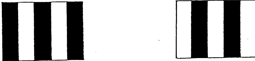
Figure 11: Change of the interference pattern when the distance between S_1 and R is changed by \lambda/4 .
