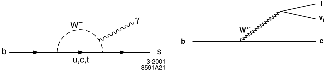
Figure 4: Example Feynman diagrams for a Penguin b \rightarrow s\gamma decay (left) and a tree level b \rightarrow c decay (right).
