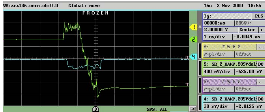
Fig. 29. Difference signals on damper pick-up during the passage of an LHC batch in the SPS ( 1\mu\text{s}/\text{div} ); the signal observed at low frequency (green line, shifted due to electron cloud) and the downmixed signal sampled at 120 MHz (blue line, without final offset). (Courtesy W. Hofle, 2000)
