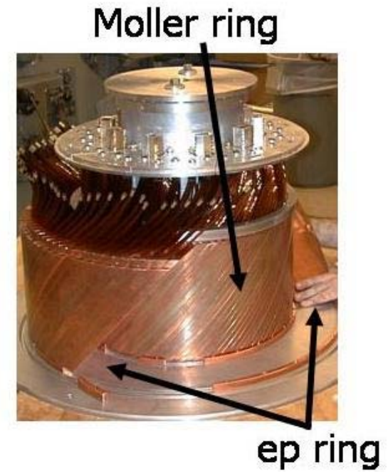
Figure 5.2: Photo of the Møller detector during assembly. In this orientation, the beam would strike the detector from underneath. Visible are the copper slabs and the fibers, which lead upward to a point where the lightguide will be attached.
