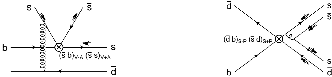
Figure 5-23. Quark helicities in \overline{B} \rightarrow \phi K^* matrix elements: the hard spectator interaction for the operator (\overline{s}b)_{V-A}(\overline{s}s)_{V+A} (left), and annihilation graphs for the operator (\overline{d}b)_{S-P}(\overline{s}d)_{S+P} with gluon emitted from the final state quarks (right).
