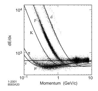
Figure 3.2: Measurement of dE/dx in the DCH as a function of track momenta.
