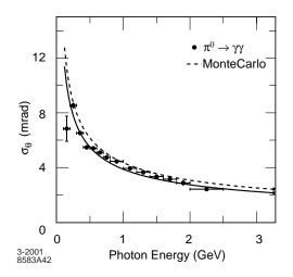
Figure 3.6: The angular resolution of the EMC for photons from  $\pi^0$  decays. The solid curve is a fit to an empirical equation.
