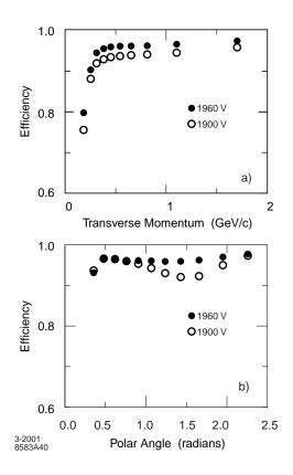
Figure 3.3: Track reconstruction efficiency in the DCH as a function of a) transverse momentum, b) polar angle.
