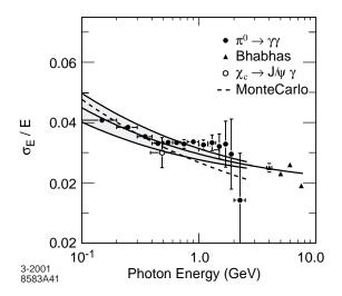
Figure 3.5: The energy resolution for the EMC measured for photons and electrons from various processes. The solid curve is a fit to an empirical equation and the indicated area denotes the rms error of the fit.
