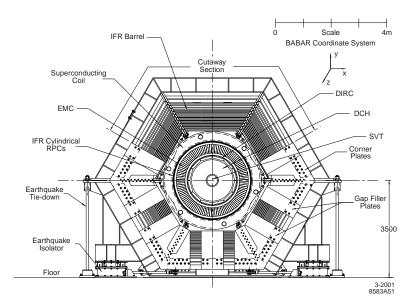
Figure 3.1: A cross-section of the *BABAR* detector. The five detector components are labeled, SVT, DCH, DIRC, EMC and IFR, listed from the inside out.
