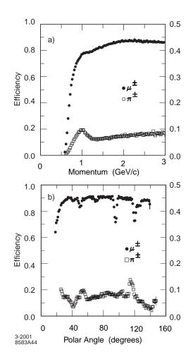
Figure 3.7: Muon efficiency (left scale) and pion misidentification probability (right scale) as a function of a) the laboratory track momentum, and b) the polar angle (for 1.5 momentum), obtained with loose selection criteria.
