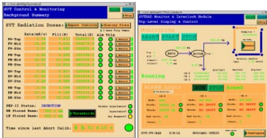
Figure E.3: Sample EPICS screenshots. The left hand screen shows summary information for each diode, including dose rates, integrated dose, alarm status, and trip alarms, and links to more detailed expert controls. The right hand screen shows the more primitive EPICS proxy for the SVTRAD module, whose ADC samples and configuration information are used to form the radiation dose rates in the summary panel on the left.
