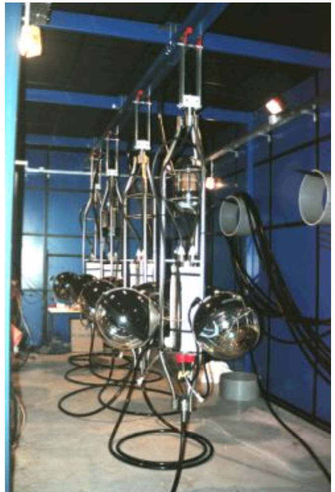
Fig. 16 Titanium optical module support frames for 'triplet' stories of the Antares detector
