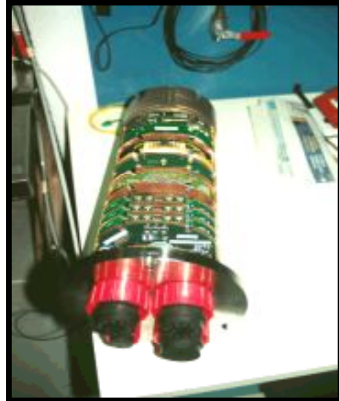
Fig. 25 Local electronics container (titanium) for the three optical modules of an Antares “triplet”
