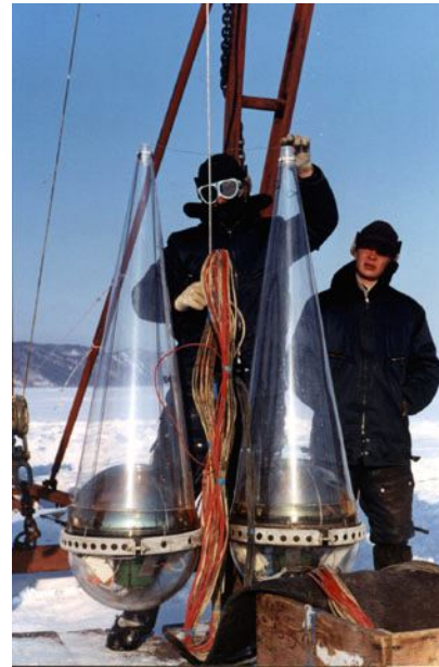
Fig. 13 Upward-looking Quasar-type optical modules from the Lake Baikal array. (Anti-sedimentation cones fitted.)
