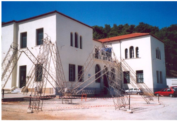
Fig. 15. Partially folded titanium frame of a Nestor 'floor' (at Nestor Institute, Pylos)
