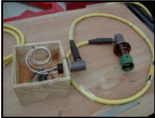
Fig. 21 Hybrid underwater-mateable connector receptacle by Ocean Design Inc.
