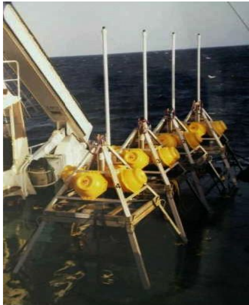
Fig. 26 Deployment of the acoustic transponders of the Antares long baseline survey system
