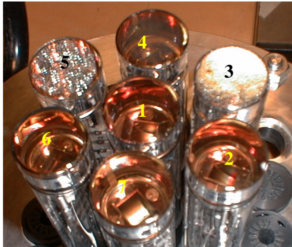
Figure 7. Appearance of seven PMTs, as the beginning of the corrosion test. One can see four “clear” PMTs on the bottom, two “frosty” on each side, and one “milky” at the top right-hand side.
