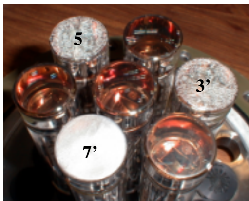
Figure 9. The same PMTs as in Fig. 7, after the second immersion in hot water for 30 days (equivalent to 12 months at 28°C). Scratches appeared on four “milky” PMTs, and edges of the “frosty” PMT # 5 also became “frosty.” It is the first immersion for PMT #3’ and 7’.
