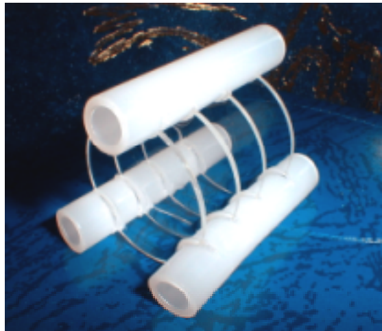
Figure 14. Four B53 glass window coupons with supports.
