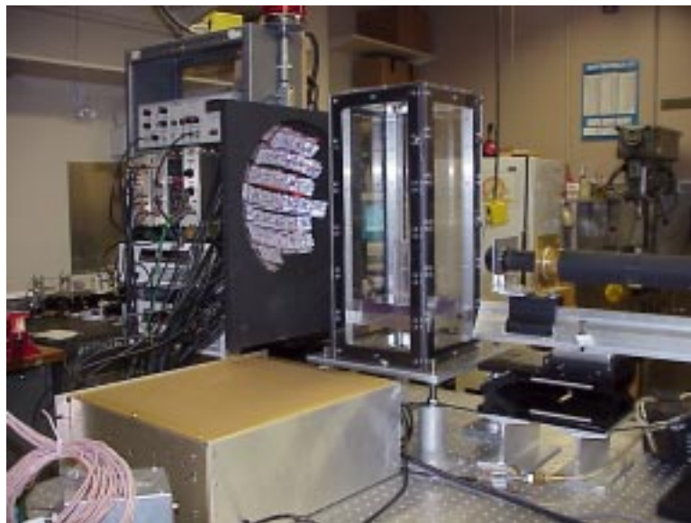
Figure B.1: A picture of the LED strobe backlighting the falling drops in the main chamber.
