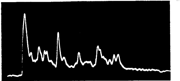
Fig. 11 - Example of a single event in one stage (4.7 cm of drift). Ne + 5% C_2H_6 , v_d = 2.2 cm/ \mu s. 10 ns sampling interval.
