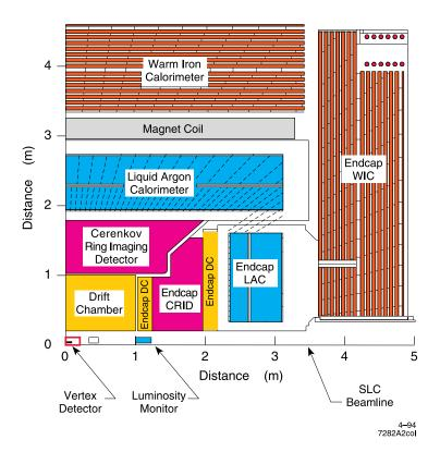
Figure 2: A quadrant view of the SLD detector.
