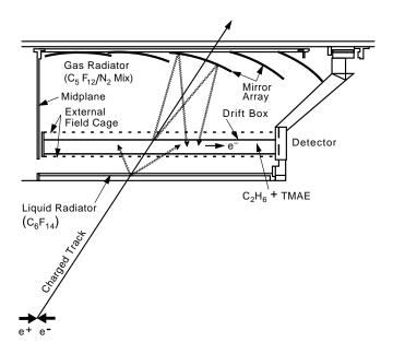
Figure 3: Cross-section view of one CRID quadrant.
