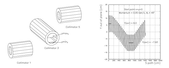
Fig. 9. The arrangement of the collimators that are used to eliminate high energy negative and all positive particles from the beam is shown on the left. On the right is a plot of the drift of a particle perpendicular to the plane of the transport as a function of the total path-length. It drifts down in the first half of the transport solenoid and back up in the second half.
