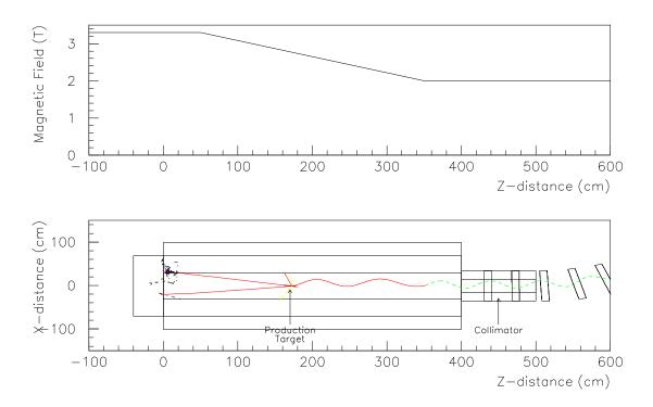
Fig. 8. Schematic drawing of the production solenoid, on which a simulated event with a proton interaction is superimposed, producing a  $\mu^-$ . The incident proton beam enters from the right. Above the drawing is a plot of the axial component of the magnetic field in this region as a function of z.
