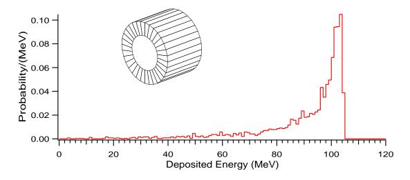
Fig. 11. The energy response of the electron trigger calorimeter for 105 MeV electrons. The inset shows the geometry of the detector. Each azimuthal slice is divided into  $\sim 50$  tiles.
