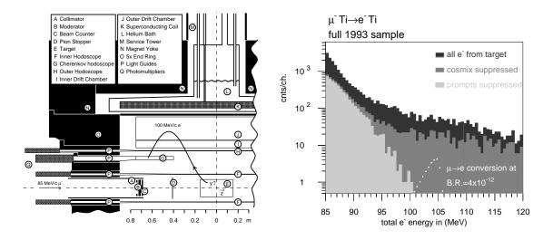
Fig. 4. A cut view of the SINDRUM2  $\mu^- N \rightarrow e^- N$  apparatus is shown on the left. The histogram shows detected electron energy distributions; the lightly shaded contribution is after all cuts have been applied and consists primarily of electrons from muon decay in orbit. The medium shaded region contains background removed by vetoing on events which are in time with a signal in the beam counter, and the heavily shaded area contains events removed by cosmic ray cuts.
