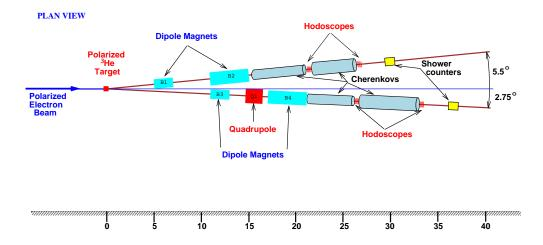
Fig. 7. Schematic plan of the E154/E155 spectrometers.
