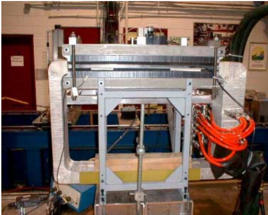
Figure 10.1. Apparatus for magnetic field quality measurements.
