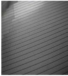
Figure 2.2.3 An enlarged view of a diced crystal analyzer Ge(733) [Isaacs, Abbamonte et.al.][11].
