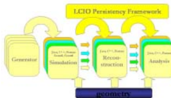
Figure 1: Schematic overview of the simulation software chain. LCIO defines a persistency framework for the simulation and reconstruction stages. It is suited to replace the plethora of different data and file formats currently being used in linear collider simulation studies (denoted by the small arrows).
