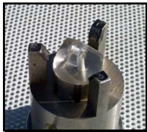
Fig. 18 Glass-cube with vacuum holes
