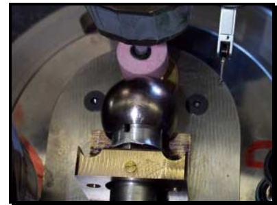
Fig. 12 Grinding spherical housing
