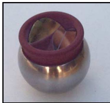
Fig. 11 Air-cube with Rulon® collar
