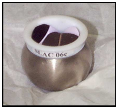
Fig. 10 Air-cube with Teflon® collar
