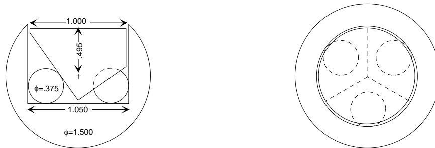
Fig. 3 Corner-cube installed in 1½ inch ball
