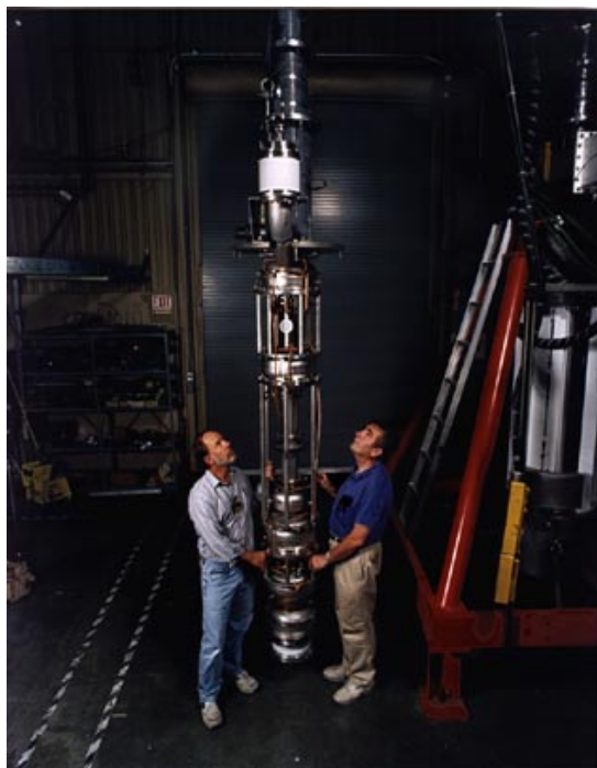
Figure I: 500 kW, 400 MHz LHC Klystron
