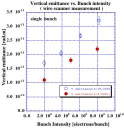
Figure 2: Recent results of emittance measurements using wire scanners at the EXT.
