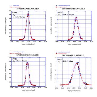
Figure 3: Vertical wire scans in the EXT, using W filaments with  $10\mu m$  diameter.
