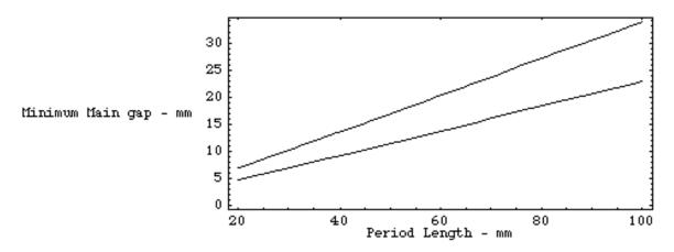
Figure 3: The minimum main gap allowed by the demagnetization of ferrite magnet material, with Br = 0.37 T and Hc = 325 kA/m. The upper curve is for the case of counterforce and main arrays of equal width and the lower curve is for counterforce magnets twice as wide as the main magnets. Both curves assume magnets with square cross section.
