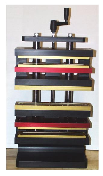
Figure 6: Prototype counterforce system. The black jaws hold the main magnets (gold keepers in center) and the moving counterforce magnets (gold keepers at bottom and top). The red fixtures hold the stationary counterforce magnets. The lead screw is 12.7 mm diameter with a pitch of 0.787/mm. The crank handle is 65 mm from axis to handle axis.
