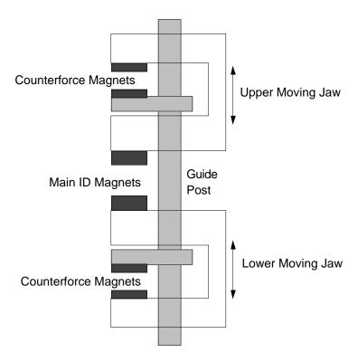
Figure 1: Schematic End View of an insertion device, showing two moving jaws with main ID magnets and counterforce magnets mounted on them. There are also two fixed rows of counterforce magnets, opposite each set of moving magnets.
