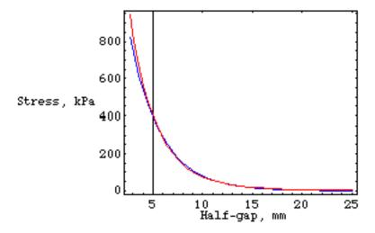
Figure 5: Stress curves for hybrid (red) and pure ferrite counterforce (blue) magnets. This fit was achieved with  $\Delta=7.7$  mm,  $\lambda_c=0.8$   $\lambda_m$  and equally wide main and counterforce magnets.
