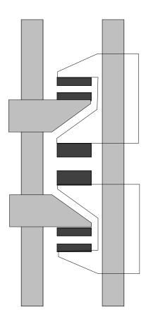
Figure 4: An alternative design, where the stationary counterforce magnets are held on a separate pillar, with supports shaped to allow more compact jaw profiles.
