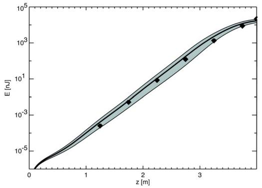
Figure 4. Energy vs. Distance. GENESIS simulation compared to measured data different that in Fig. 1. Gray area indicates a one sigma shot noise fluctuations due to different seedings in GENESIS.
