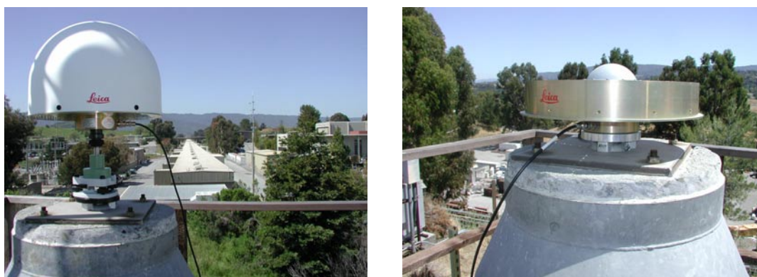
Figure 1 Station SLAC M40 at the end of the LINAC housing with the Leica AT-504 choke ring antenna in the setup before (left) and after (right) the mount change.
