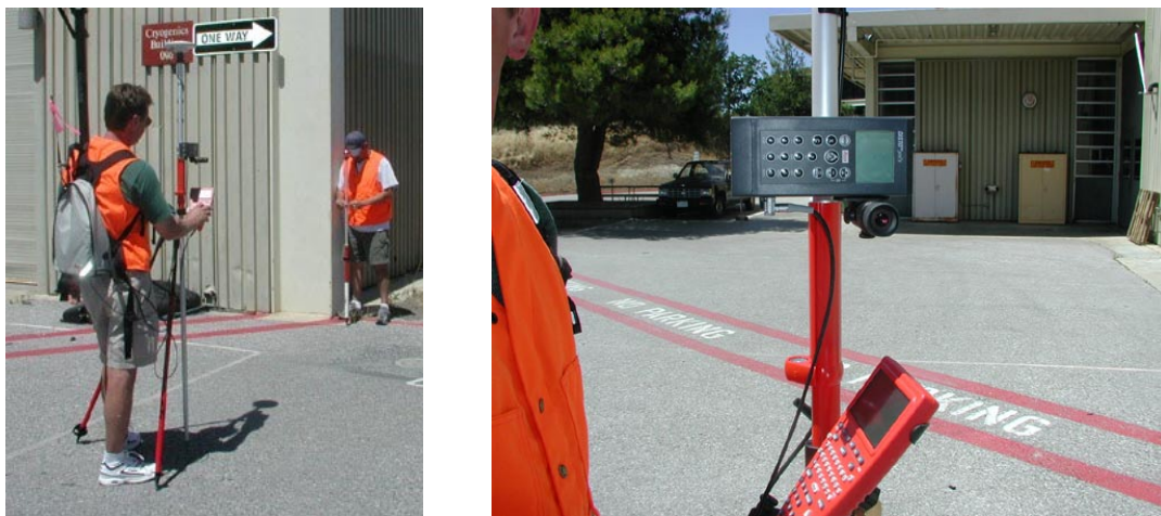
Figure 2 Leica SR-530 rover unit with AT-502 antenna and DISTO Pro A distance meter employed in a survey at SLAC.
