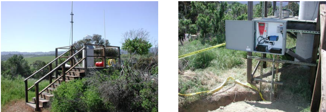
Figure 3 SLAC M40 with the wooden deck surrounding the 60 cm diameter concrete pillar and the weatherproof box for the Leica System 530 base receiver.
