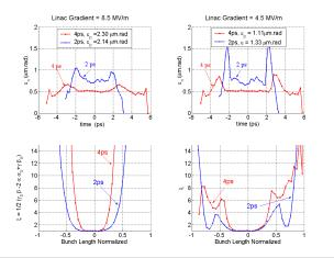
Figure 3. Slice emittance and matching parameters.
