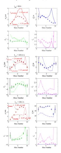
Figure 4. Slice emittance, Twiss parameters and matching parameters for a 200pC, 3 ps fwhm bunch for 3 different solenoid values; experiment (circles) and Parmela (lines), both for 10 slices.
