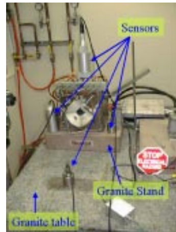
Figure 7: EM quadrupole vibration measurement setup.
