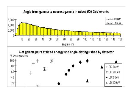
The upper plot illustrates the environment in 500 GeV ee->qq (q=u, d, s, c or b) events with a boost less than 0.2c to eliminate forward events due to ISR down to the Z pole. For each final
