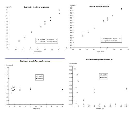
As stated above the ideal calorimeter will be able to isolate neutral particle showers. We have studied the capability of the S and L detectors to isolate photon showers. The following plots show the results.
