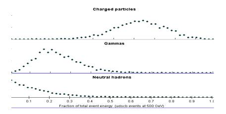
The ideal detector will be able to reconstruct the high mass jet-producing particle by reconstructing each individual particle in the jet. Can calorimetry meet this challenge for the neutral particles? The situation regarding gammas and neutral hadrons, the two categories of neutrals, is somewhat different and we will discuss each case.
