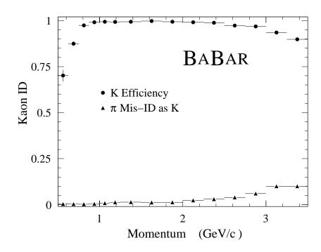
Figure 11: Efficiency and misidentification probability for the selection of charged kaons as a function of track momentum, for a particular choice of particle selection criteria. The data use  $D^0 \to K^- \pi^+$  decays selected kinematically from inclusive  $D^*$  production.
