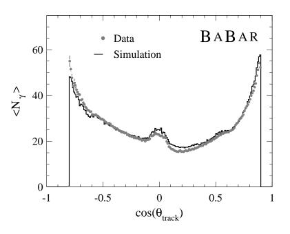
Figure 7: Number of detected photons versus track polar angle for reconstructed tracks in di-muon events compared to Monte Carlo simulation. The mean number of photons in the simulation has been tuned to match the data.
