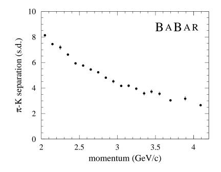
Figure 10: DIRC  $\pi$ -K separation versus track momentum measured in  $D^0 \to K^- \pi^+$  decays selected kinematically from inclusive  $D^*$  production.
