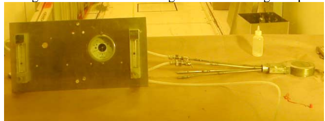
Figure 1: SLC Positron Target Leak Checking Setup
