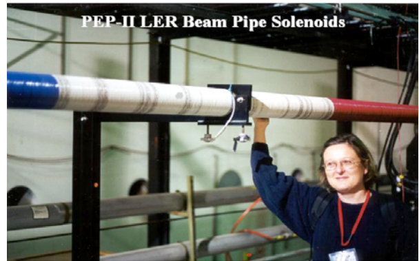
Figure 7: Straight section solenoid windings.
