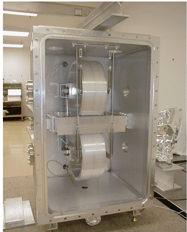
Figure 5: Consumable spoiler prototype
