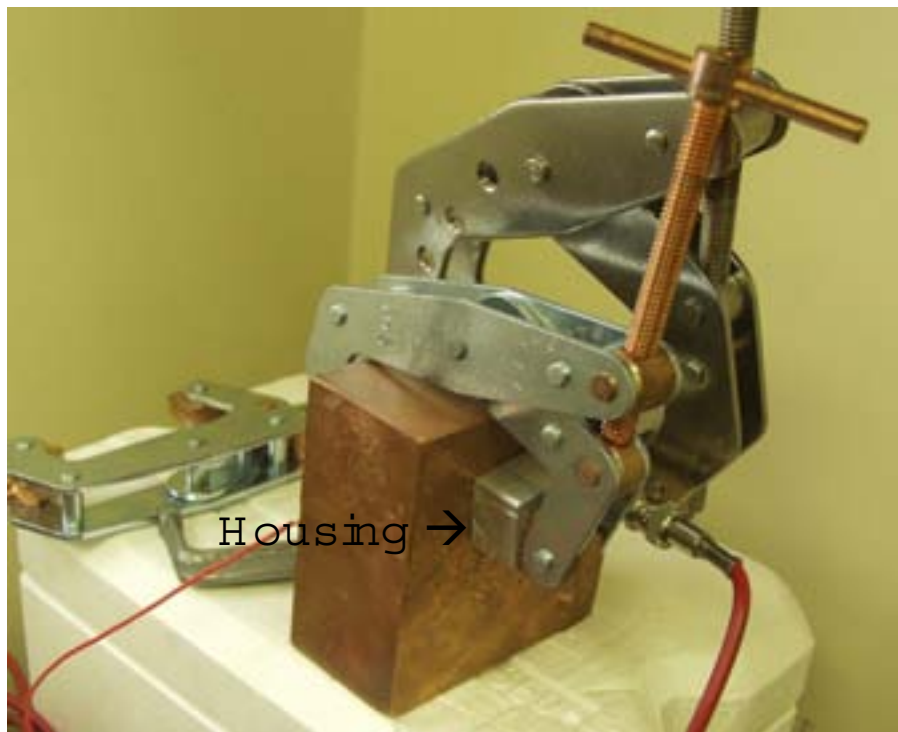
Figure 2. The new housing for the spark gap, clamped to the block.
