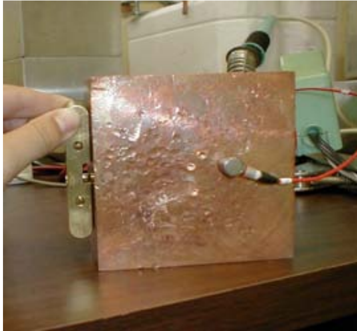
Figure 1. Original design for the spark gap housing. Note the gap between the housing and block, through which energy was being lost.
