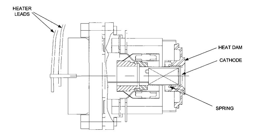
Figure 5. A close up of the cathode assembly enclosure.
