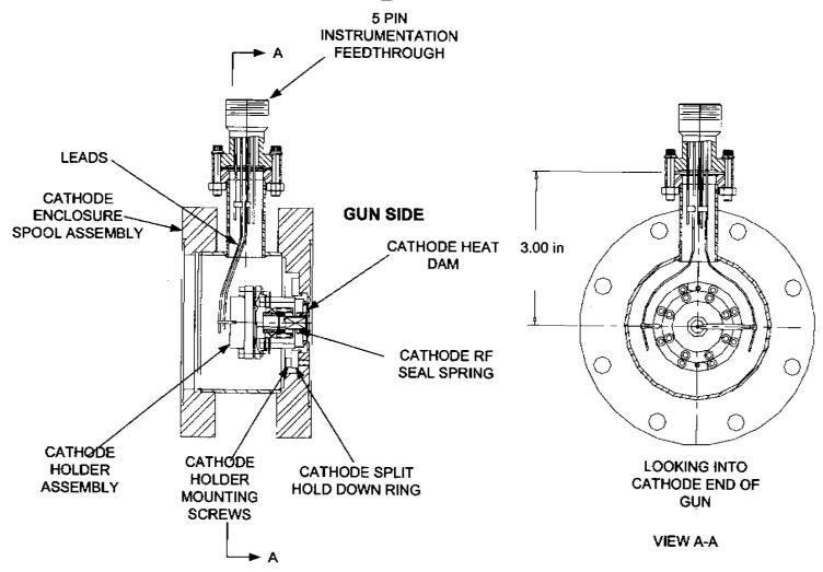
Figure 4. A schematic of the cathode assembly
