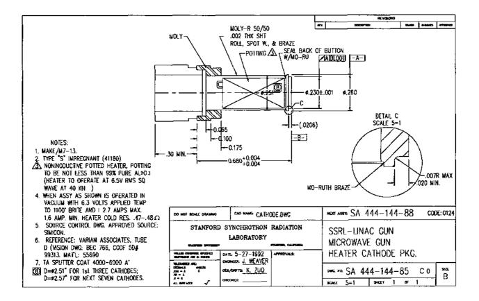
Figure 3. This is an SSRL Autocad drawing of the cathode, also known as the heater cathode
