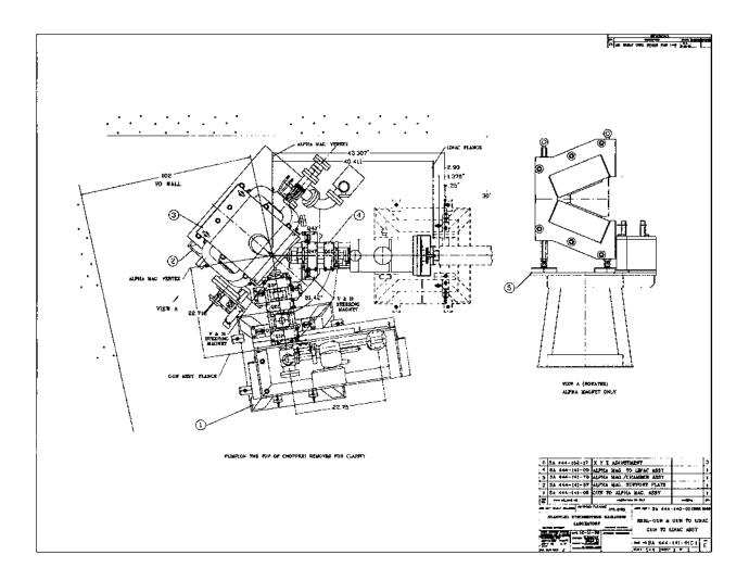
Figure 2. A SSRL Autocad schematic of the Gun to Linac (GTL) setup. This includes the RF gun, a series of quadrupoles, and the alpha magnet.
