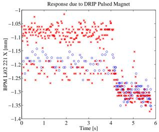
Figure 3: Pulsed magnets don't fully recover at 120 Hz. The transition from "75Hz" (60+15) to 116 Hz occurs at 4 sec. The 200  $\mu$ m difference could not be fixed yet, but is reduced to only 30  $\mu$ m at the end of the linac.
