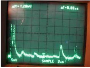
Figure 4: Beam loss along the linac.
