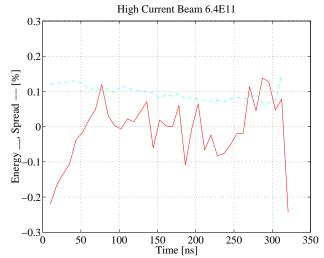
Figure 5: Energy and energy spread along the pulse. The finite rise time of the pulse creates a low energy tail.
