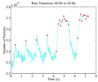
Figure 2: Different rates create different intensities. The rate changed from 60 Hz (58Hz for E-158, 2Hz for PEP-II) to 20 Hz for E-158 at around 4.5 and 6.5 sec. The pulse after PEP and the 20 Hz are marked in red (\*). The higher intensities reduce the beam energy.
