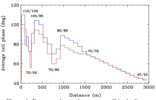
Figure 1: Betatron phase advance per cell in the linac.
