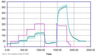
Figure 6. Be bellows temperature rise (deg C) (upper curves right) with heater current (center) with (left) and without (right) 5 CFM air cooling during lab bench tests.
