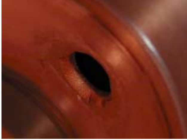
FIG. 22: A picture of the high-power coupling aperture of cavity 1 after the first high-power test. The aperture has been rounded in the direction of the magnetic field. The electric field has caused pitting to occur on either side of the aperture at right angles to the rounding.
