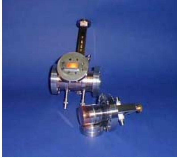
FIG. 4: A picture of the cavity body with one endcap shown on the outside. The water-cooling pipes can be seen on the bottom of the cavity body.
