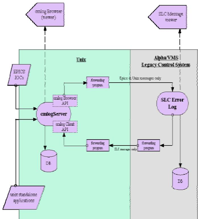
FIGURE 2.1: simple cmdSrv example configuration.
