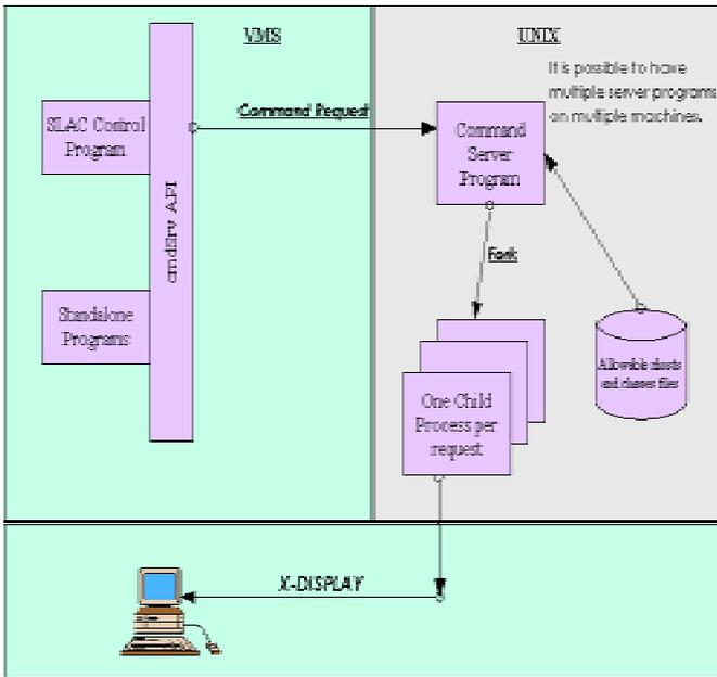
FIGURE 2.1: simple cmdSrv example configuration.
