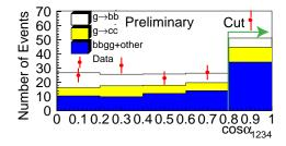
Figure 2: The distribution of the cosine of angle between the plane  $\Pi_{12}$  formed by jets 1 and 2 and the plane  $\Pi_{34}$  formed by jets 3 and 4, for data (points) and Monte Carlo (histogram). We reject  $|\cos \alpha_{1234}| > 0.8$
