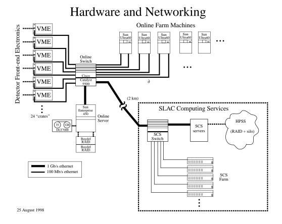
Figure 1: Diagram of the BABAR online computer farm architecture showing the VME PowerPC frontend computers, the online farm of Sun UltraSPARC computers, the Sun Enterprise 450 server with the intermediate store disk array and the SLAC computer center farm connected using Cisco Catalyst 5500 switches.
