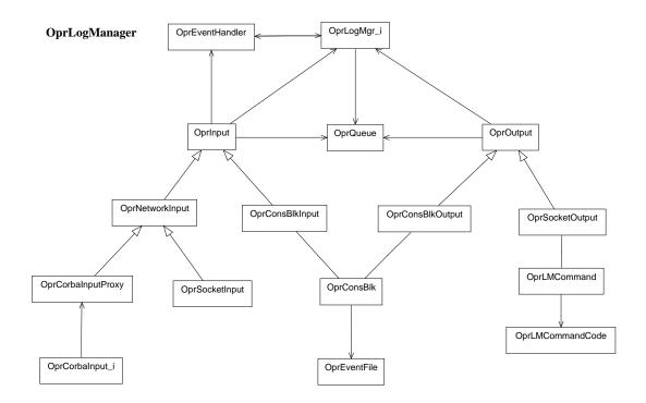
Figure 3: Logging Manager simplified class diagram.
