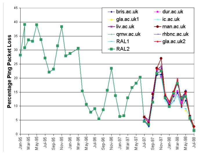
Figure 1: Performance between Monitoring Sites on ESnet and sites in the UK. Note the drop in packet loss (i.e., improved performance) in August '95, April '96 and July '97 corresponding to increased bandwidth on each occasion. Also note similar improvements in August and December corresponding to University holidays.
