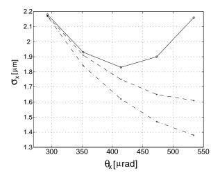
Figure 2: Horizontal beam size  $\sigma_y$  at the SLC IP as a function of angular divergence  $\theta_y$ . Curves (solid), RMS, and (dashed), with proper integration, are for the 1996 optics. The dot-dashed is for 1997 optics.
