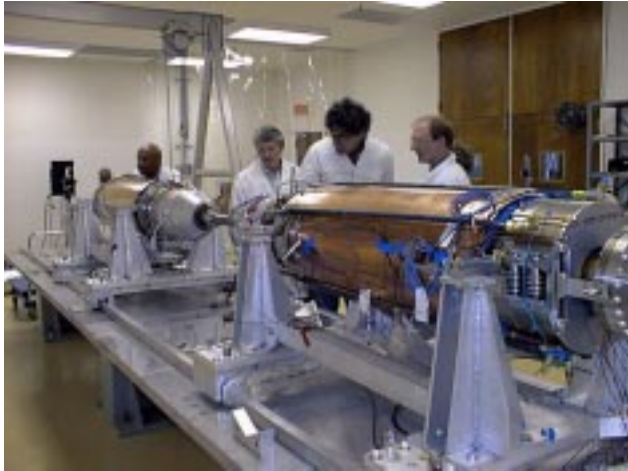
Figure 7. Assembled beamline from Q1 to Q1 before being inserted into the support tube.
