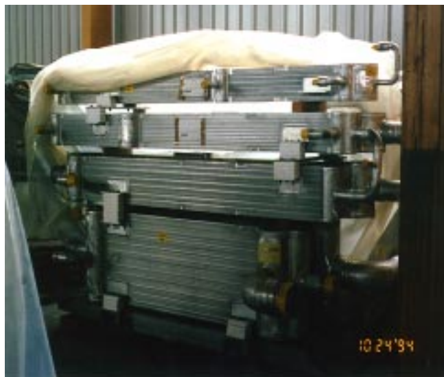
Figure 2 Heat Exchanger Train
