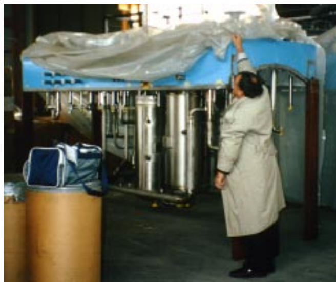
Figure 1 Cold box/valve box with components
