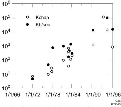
**Figure 4** Evolution of the number of detector signal channels with time, indicating growth of collider detector instumentation capability over the last 24 years. The open circles indicate the number of electronic instrumentation channels in thousands. The closed circles indicate the design data rate in kilobytes per second to permanent storage. The date is that of the detector proposal or Technical Design Report; e<sup>+</sup>e, pp, and pp detectors are included.
