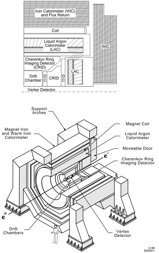
Figure 5 Cutaway and quadrant view of the SLD detector.
