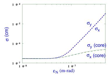
Fig. 9. Variation of the rms IP beam sizes and the rms 'core' beam sizes at the first IP focal point (the 'core' is obtained by removing fliers outside  $\pm 9\sigma$ ) versus the normalized beam emittance.
