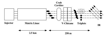
Fig. 13. Schematic (not to scale) of a W-band final focus with multiplexed collisions, crossing angle, crab cavities and charge compensation ('multiplexed collisions').
