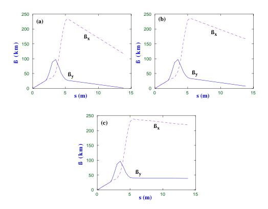
Fig. 12. Horizontal and vertical beta functions calculated from the interaction point backwards through the final triplet for an energy deviation relative to the design optics of (a) -10%, (b) -5%, and (c) 0%. The IP beta functions are held constant at  $\beta_{x,y}^* \approx 150 \ \mu\text{m}$ . The IP is on the left in these figures.
