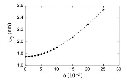
Fig. 6. Energy bandwidth for the final-focus optics of Fig. 5, as obtained from a tracking simulation with the program MAD.<sup>11</sup>
