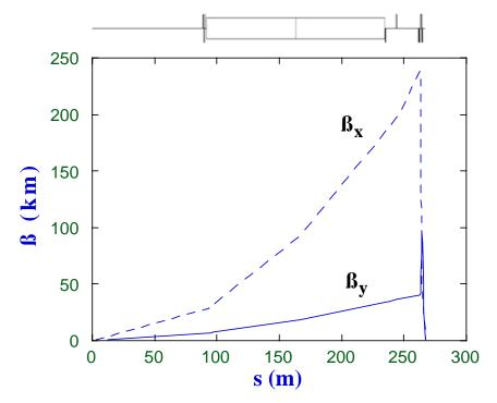
Fig. 5. Final-focus optics for a W-band linear collider, with a total length of 270 m. The IP is on the right in this figure.
