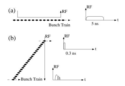
Fig. 2. Schematic of bunch trains and rf pulses: (a) in a conventional traveling-wave linac; (b) in a switched matrix accelerator.
