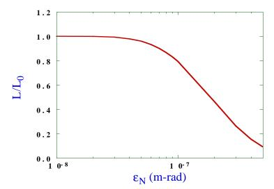
Fig. 10. Relative luminosity reduction at the first IP focal point due to the Oide effect versus the normalized beam emittance. Luminosity is computed using area-weighted charge allocation on a Cartesian grid.
