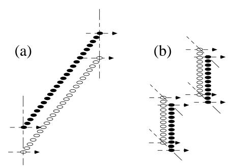
Fig. 3. Schematic of timing patterns for two different collision schemes: (a) for multiplexed collisions; (b) for cluster collisions. The black and open ellipses represent electron and positron bunches, respectively, which are later combined to form neutral beams.
