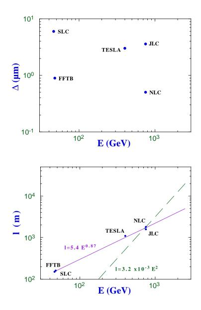
Fig. 4. Energy scalings exemplified by 5 different final-focus designs: (top) orbit-sextupole sensitivity  $\Delta$  vs. beam energy; (bottom) system length vs. beam energy.
