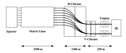
Fig. 11. Schematic (not to scale) of a W-band final focus combining groups of 12 bunches into superbunches, which are charge-compensated and collided head-on ('cluster collisions'). There is one common interaction point for every 12 linac bunches.
