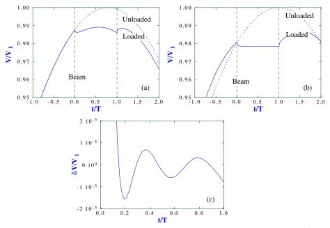
Fig. 7. Loaded and unloaded voltage waveforms for a wakefield parameter  $\nu = 0.5$ : (a) in a conventional single frequency linac, with a total rms energy spread of  $\delta_{rms} \approx 10^{-3}$ ; (b) in a two frequency linac, with  $\delta_{rms} \approx 1.6 \times 10^{-4}$ ; (c) in a three frequency linac, with  $\delta_{rms} \approx 2.5 \times 10^{-6}$  excluding the first 10% of the beam (shown here is the difference from the average voltage; note the magnified scale).
