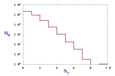
Fig. 8. Histogram of number of photons emitted per electron in the final doublet. The first bin corresponds to 0 photons radiated. The total number of electrons sampled in the simulation was  $N \approx 3.3 \times 10^5$ .
