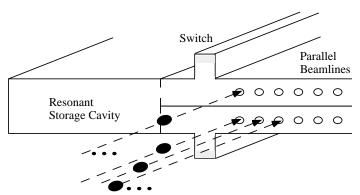
Fig. 1. A switched matrix linac consisting of 25 parallel positron beam lines, situated below 25 parallel electron beam lines.
