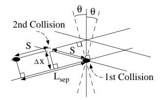
Fig. 14. Multiplexed collisions with a crossing angle.
