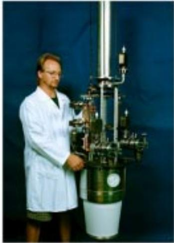
**Fig. 15** 50-MW PPM X-Band Klystron
