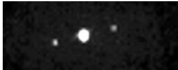
Fig. 9 Light pattern observed in lobe-producing bars after a single pass through the bar.
